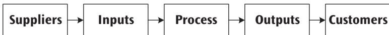
Exhibit 2-1. SIPOC diagram. Typically under each part of the diagram you can list the processes and activities involved.
